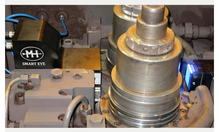
Smart eye consists of a portable camera unit, protective case with built in high capacity battery pack and screen, bench with screen and a collimated LED backlight source especially developed for optics. The portable camera is a high-resolution camera which is IP67 protected to withstand the hostile environment of a rolling mill, and the same camera can be used on the bench as well as in the wire rod block.
